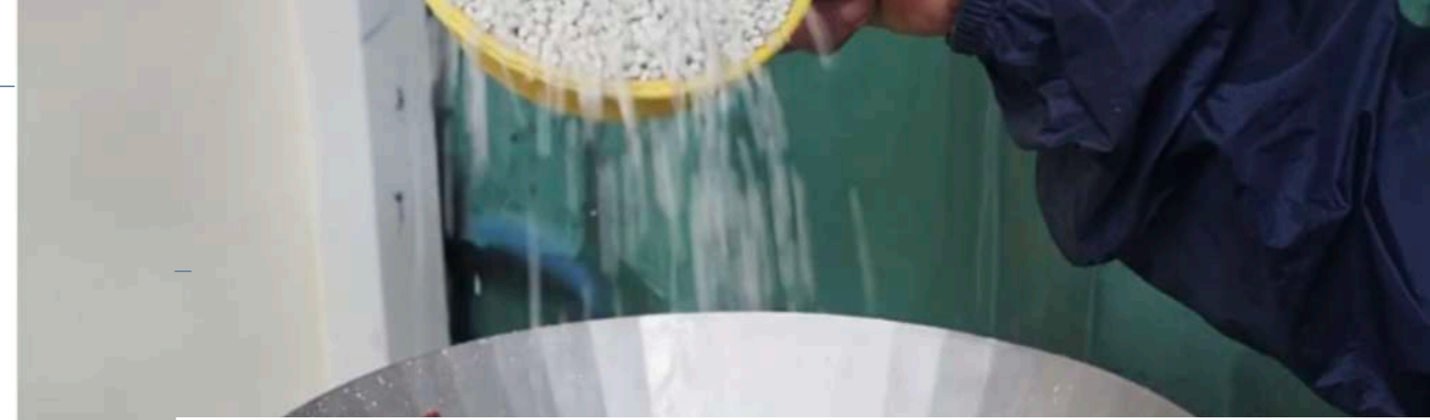
Figure 62 Loading shredded plastic into feed hopper
