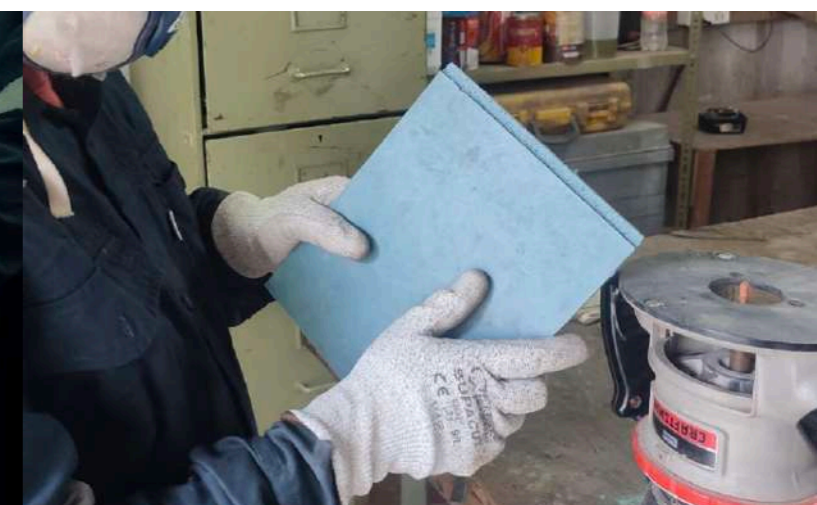
Figure 74 Making shallow passes for controlled cutting depth
